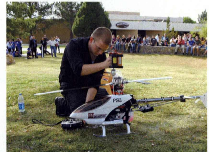
Above: Jesse McAvoy demonstrates the autonomous helicopter serving as a base platform for visual-based flight control
