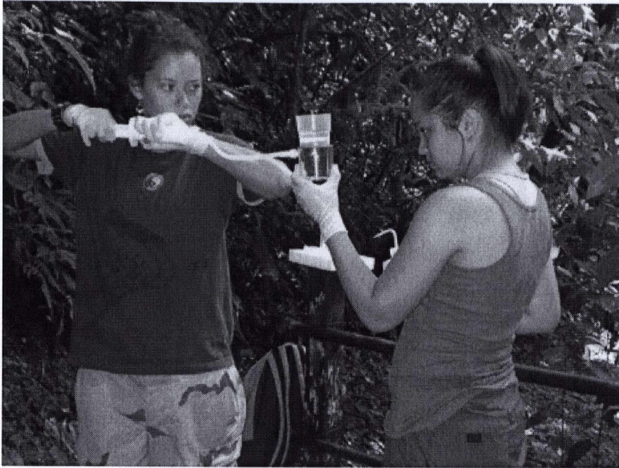
Photo 2. Trisha Soares (left) and Anna Lee Herrera (right) run a water sample through a filter in search of aquatic microbes.
