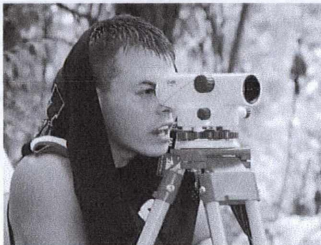
Nicolai operating a compensator type, automatic engineers level to survey a river cross-section on a restored section of the Jocko River near Arlee. The work conducted by Nicolai is being performed as part of a collaborative study between the University of Montana and Salish Kootenai Colleges' Department of Natural Resources, focusing on large river ecosystems. (courtesy photo)
