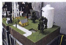
Customized, scaled model of a city water supply system used by NSF Cyber Corps students to test operating software weaknesses.
