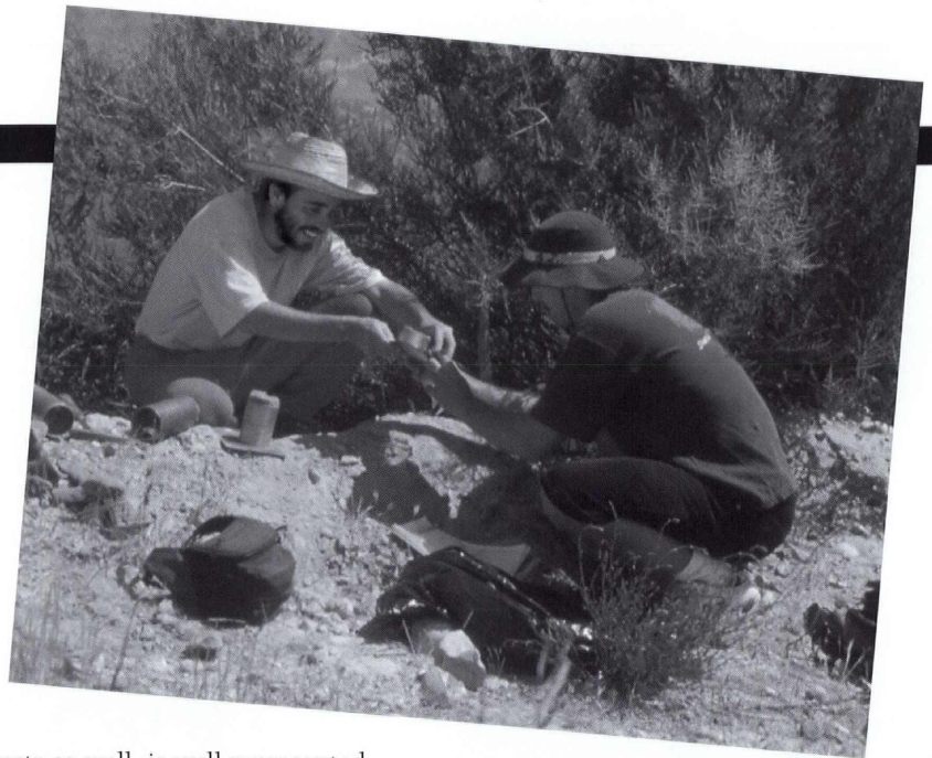
Diego Pedreros (left) and Jason Leroy (right) collecting soil samples in the Santa Monica Mountains. The soil samples were collected to measure soil moisture, needed for interpreting Synthetic Aperture Radar data acquired the same week on April 28, 1998. Leroy was an undergraduate in geography.
