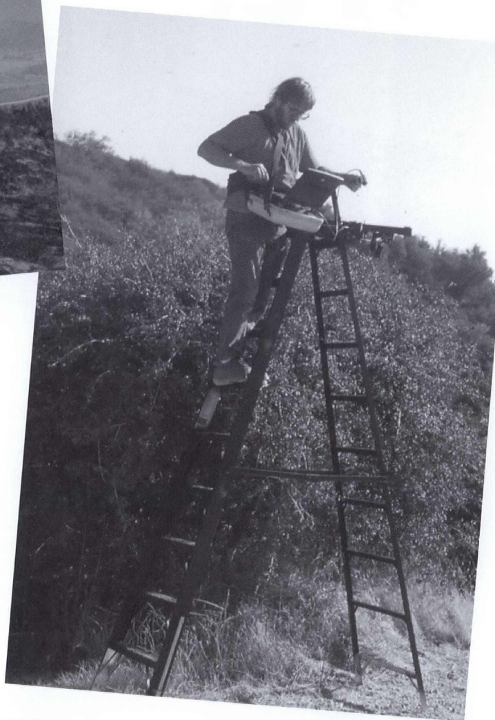
Dar Roberts collecting reflectance spectra from chaparral. The spectra are collected using a field spectrometer that samples from 350 to 2500 nm at 2 nm intervals. The spectra are used to help interpret airborne and spaceborne data. A three meter tall ladder, with leg extenders for steep slopes, is used to enable us to measure spectra above tall shrubs.
